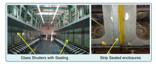
Figure 2 – The spinning machines equipped with BAT technologies of spinning machine
